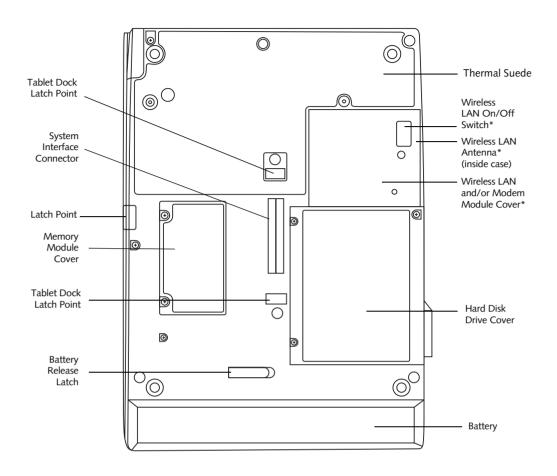
Figure 1-3 Stylistic ST4000 Series Tablet PC Features (Back View)
